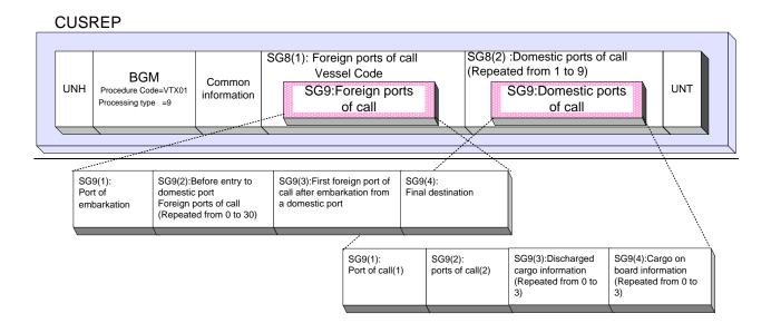
The figure above illustrates the structure of EDIFACT messages of procedure "vessel operation information registration (VTX01)." Foreign ports of call are registered in SG8 (1), and domestic ports of call are registered in SG8 (2) (maximum of 9 records).
